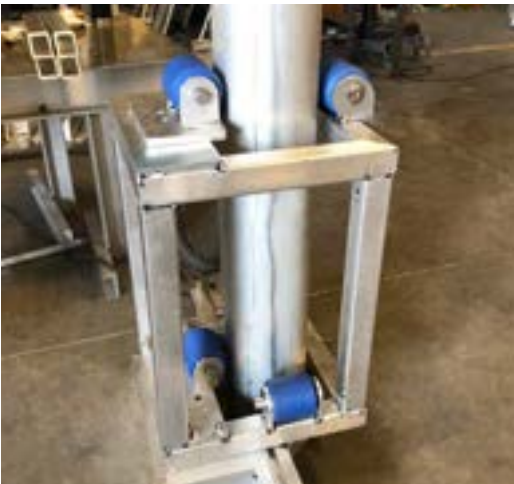
Assembled with 300 Series Stainless Steel Hardware
