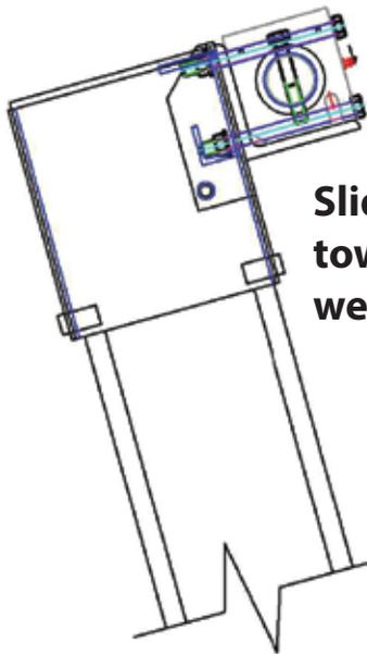
**Slide the drive head over the beam winder facing toward the water. Drill two 7/16" holes through web of I-beam and fasten with 3 1/2" bolts provided.**
