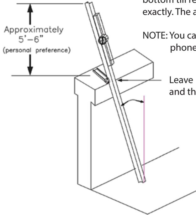
Using a Digital protractor drive or jet the I-beam into the bottom till refusal. It is important to maintain the angle exactly. The angle is pre-set when ordering the lift.
